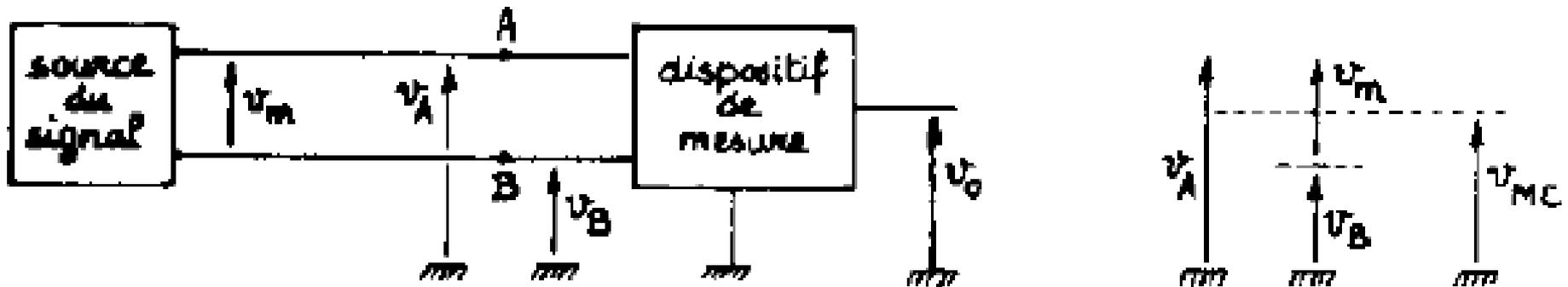
$$V_{mc} = \frac{V_a + V_b}{2} \quad V_a = V_{mc} + \frac{V_m}{2} \quad \text{et} \quad V_b = V_{mc} - \frac{V_m}{2}$$
