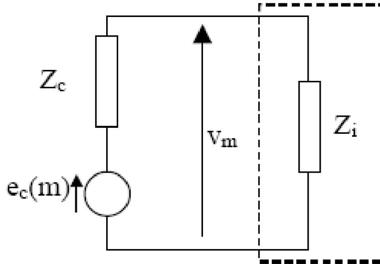
$$V_m = e_c(m) \cdot \frac{Z_i}{Z_i + Z_c} \quad \text{si } Z_i \gg Z_c \quad \text{alors } V_m = e_c(m)$$
